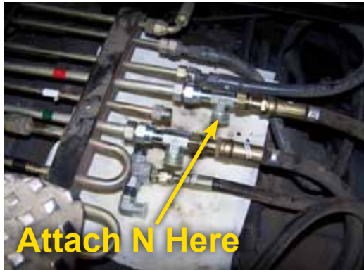
Figure 1-7: Install the Pressure Hose
