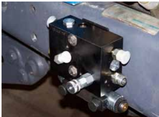
Figure 1-5: Mount the FieldPilot Valve
