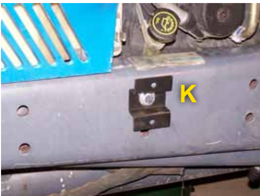
Figure 1-4: Install Mounting Bracket for FieldPilot Valve
