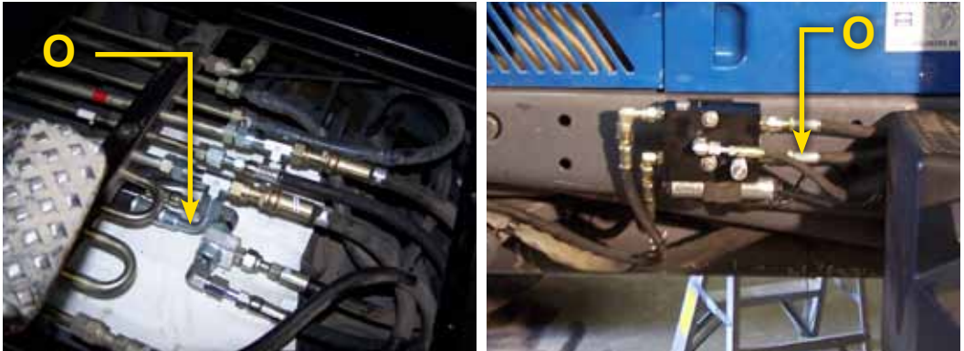
Figure 1-8: Install the Tank Hose
